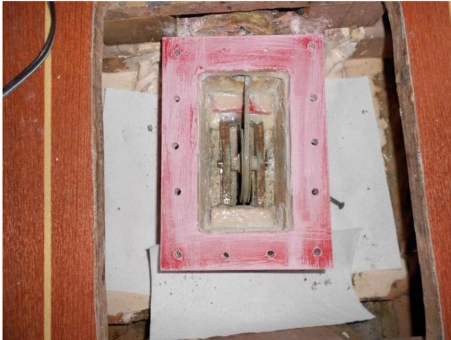
This photo shows the water tight box open with the sheave and cable exposed
