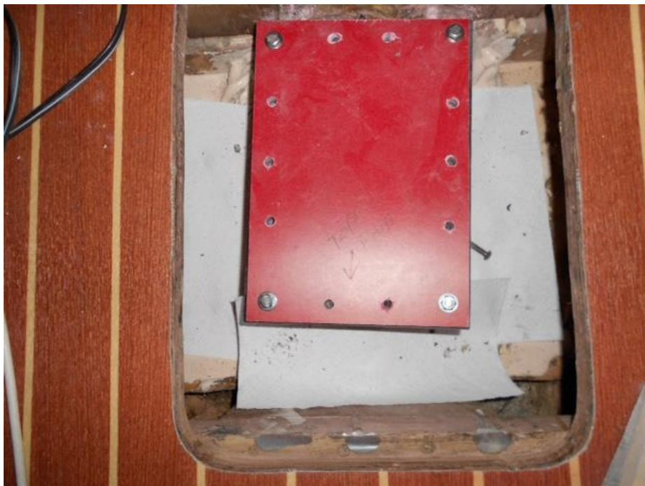
This photo shows the water tight box and lid, lid not bolted in place...this box and cover have been re-built by the owner to allow using a rubber gasket rather than caulking.
